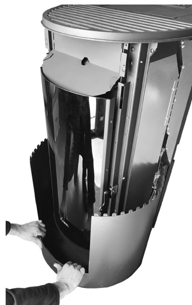
Fig. 68 - Remove the lower coque by pulling it towards you.
