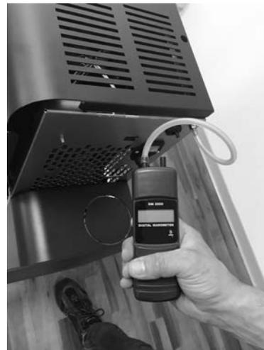
**Fig. 48 - Digital pressure switch connection**
