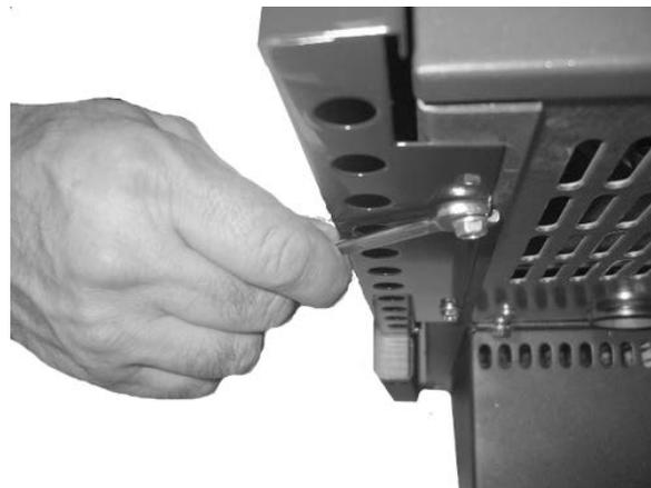
**Fig. 30 - Panels fixing**
