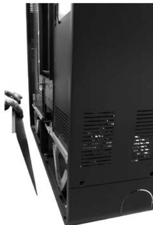
**Fig. 37 - Release of the lower bracket**
